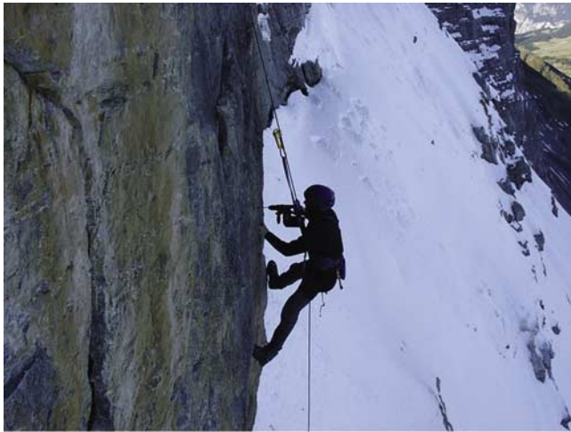
Figure 1. Installation of a rock-face temperature data logger during summer 2001.
