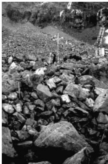
Figure 2 The surface of the Murtèl rock glacier consists of boulders varying in size from 0.4 m to several metres. The block at the front is almost 2.5 m wide. The meteorological station can be seen in the middle of the picture. Photo: S. Hanson.
